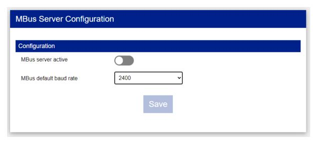
Note: "MBus server active" must only be activated if the TCP port should also be accessible from outside the device.
